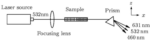
Fig. 1. Experimental set-up used in this study.
