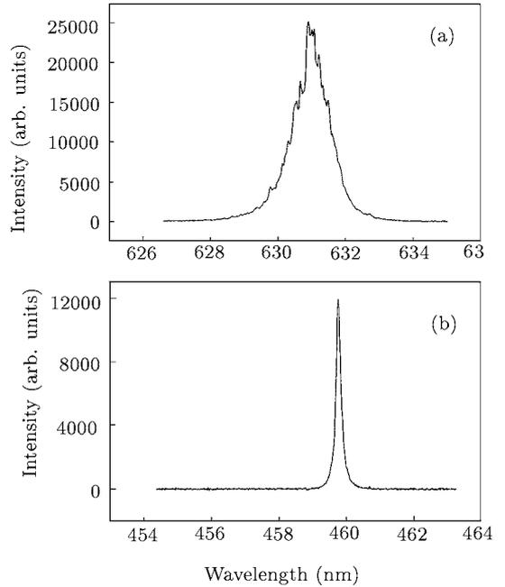
Fig. 2. Output of our experiment. The 631 nm red light was generated from the first superlattice as a signal, and the 460 nm blue light was generated from the second superlattice by adding the idler and the pump laser of the first superlattice.
