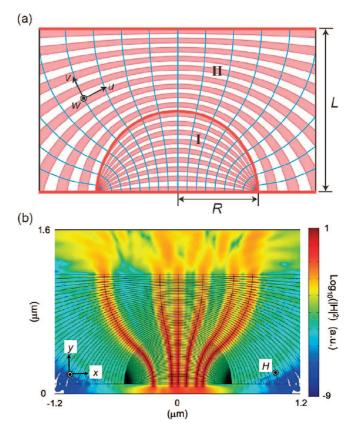
**Figure 3.** New metamaterial-based optical element: *optical transformer*. (a) Scheme of the optical transformer consisting of two domains of alternating curved layers of Ag (pink) and GaN (white). The light flows along the v axis (curved blue lines), and the interfaces between the layers comply with the u axis. (b) Magnetic field intensity profile showing subwavelength imaging and magnification of the optical transformer.
